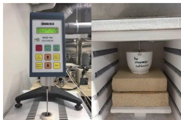
Fig.1 The apparatus for viscosity measurement
