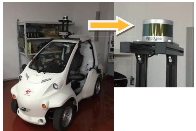
Fig. 1. Toyota's super-compact electric vehicle, COMS. The vehicle is mounted with the VLP-16 LiDAR on top, above the driver's seat. Two computers are also employed at the trunk, one for processing LiDAR data and another for using the generated information to provide control command to steer the car.
